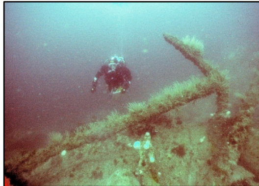
Fig 3 One of the Firebrand's four bower anchors – note the missing upper fluke.
