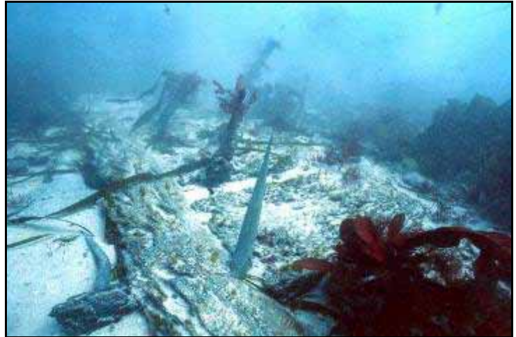
S2 Copper alloy fastenings and timber on the north side of the wreck. The hull outer planking is on the left and the frames are in the centre of the picture.
